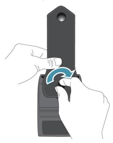
4. With the belt strap attached to the printer, place the top of the belt strap over your belt.
