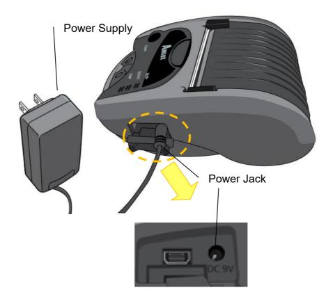
3. It takes approximately 4 hours to fully charge the battery, and the Battery LED will turn off, signifying that the battery is fully charged and ready for use.
