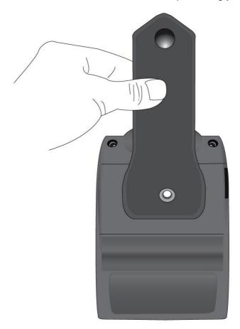
Insert the screw on the knob through the belt strap and tighten clockwise until it is fully secured.
