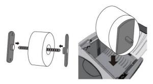
3. Pull a short length of media out of the printer. Close the media cover and press until you hear a click sound to lock it properly:
