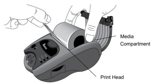
\* If the media supply roll is small, use the media shield to hold the media supply roll. For media supply rolls less than 3 inches wide, align media supply roll to slightly middle left for correct detection of media sensor. Place the media shield in the media compartment and lean it closely against the media supply roller.
